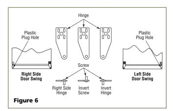
Remove bottom hinge from cabinet (four screws) and screws on opposite side of cabinet. See Figure 7.
